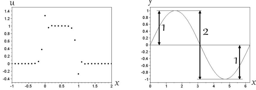
Figure 2: Algorithm with oscillations    Figure 3: The TVD of the sine function
